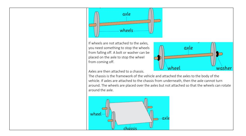
Axles not fixed to the chassis are put through holes in the chassis so that the axle can turn around. The wheels are firmly attached to the axle so they turn when the axle turns.
