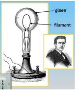
Thomas Edison invented the first practical, long-lasting lightbulb in 1879. He used an airtight glass case with a piece of looped wire (the filament) inside. When connected to a power source, the filament heated up and glowed white hot.
