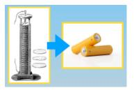
The battery was invented first, in 1800, by an Italian called Alessandro Volta. It was made by stacking discs of zinc and copper in a pile, separated by paper soaked in a saltwater solution. Volta tested the battery by giving
