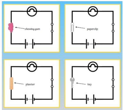
Explain that the wires are used to join the bulb, batteries and switch together in a type of loop known as a circuit. Explain that this allows the stored power from the batteries to flow through the wires and light up the bulb. Materials that allow electricity to pass through are called conductors. Which materials are not conductors?
